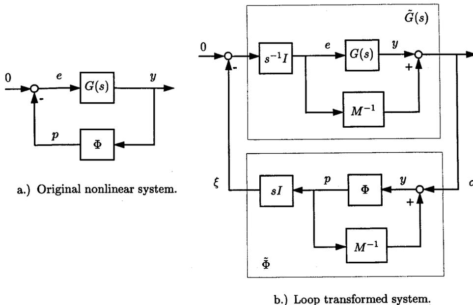
Figure 6. Non-linear system and loop transformation.
