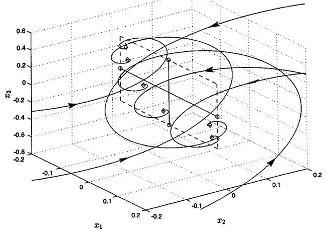
Figure 13. The stationary set E for a multiple backlash nonlinearity is a rectangular region in the  $x_1$ - $x_3$  plane.
