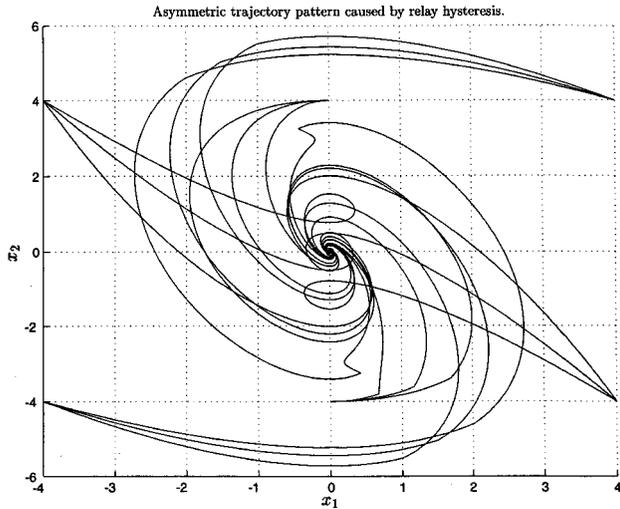
Figure 12. Trajectories are non-smooth as a result of relay switching.
