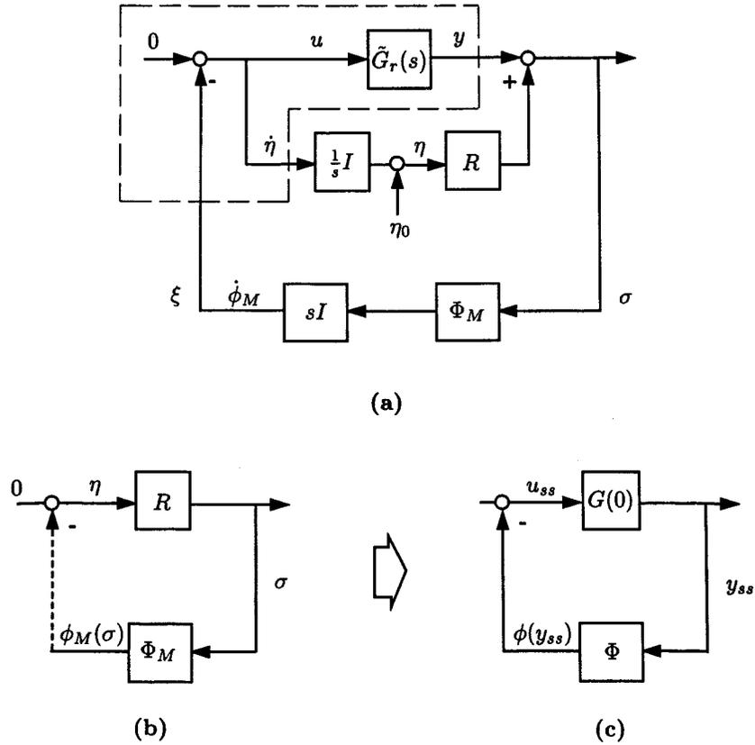
Figure 9. The condition  $\dot{V} \equiv 0$  implies steady state condition on the Popov system. The signals contained in the dashed region seen in (a) tend to zero asymptotically. In the limit, this allows reduction to the system (b), which is the transform equivalent to (c), that describes the steady state equilibrium condition (47).
