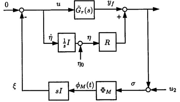
Figure 15. Popov system with initial condition response as input.
