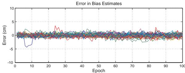
**Fig. 21:** Simulated Error in Bias Estimate During Frequent Re-Initialization, Biases Fixed with Layered Re-Initialization Algorithm
