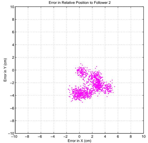
**Fig. 10:** Error in Relative Position Estimate to Second Follower Vehicle, Frequent Re-Initialization with Null Space Algorithm, Data 2
