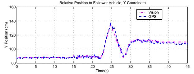
**Fig. 7:** GPS and Truth Sensor Measurements of Y Coordinate to First Follower, Re-Initialization with Null Space Algorithm, Data 1
