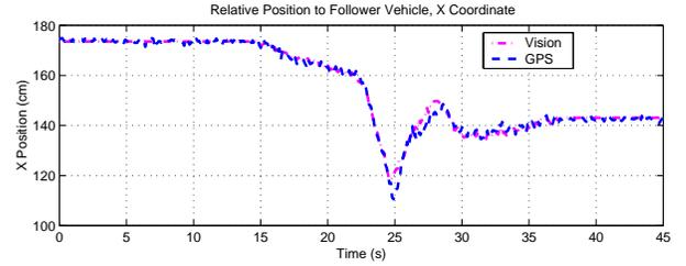
**Fig. 6:** GPS and Truth Sensor Measurements of X Coordinate to First Follower, Re-Initialization with Null Space Algorithm, Data 1
