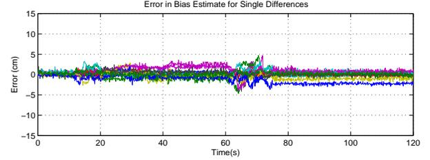
**Fig. 14:** Error in Bias Estimate for Single Difference Measurements, Frequent Re-Initialization with Null Space Algorithm, Data 2
