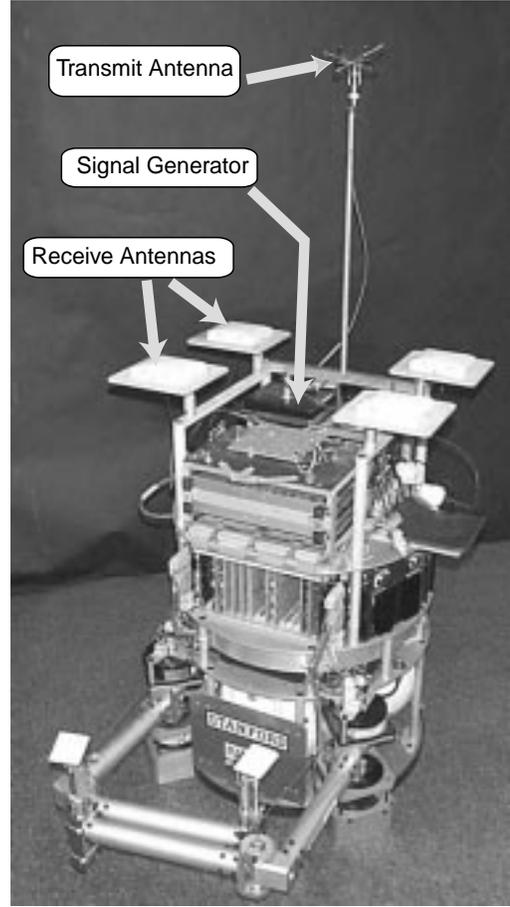
**Fig. 2:** One of Three Vehicles in the Formation Flying Testbed, Equipped with GPS Transmitter and Receiver
