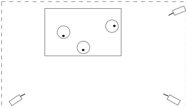
**Fig. 3:** Layout of Transmitters in GPS Testbed. Three Ceiling Mounted Pseudolites Around Perimeter, Three Robots (circles) with Transmitters Onboard.
