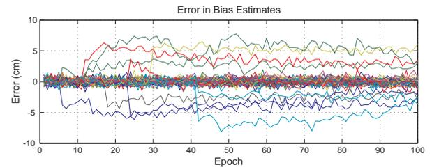
**Fig. 18:** Simulated Error in Bias Estimate for Frequent Re-Initialization with Only Null Space Algorithm
