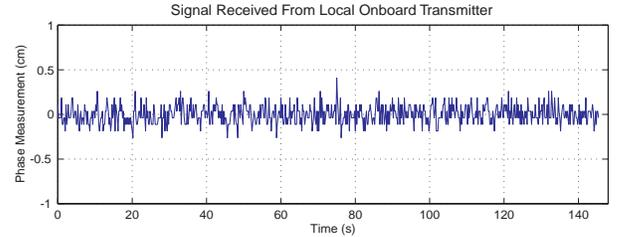
**Fig. 22:** Single Difference Measurement Between Transmitter and Receiver on Same Vehicle
