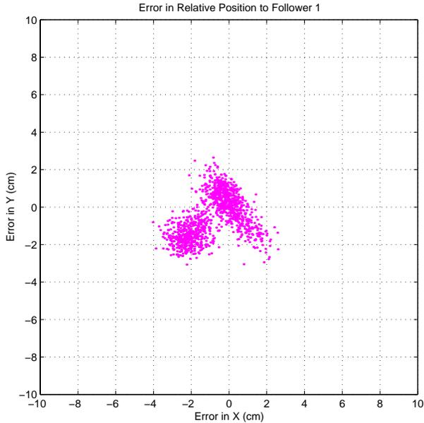
**Fig. 9:** Error in Relative Position Estimate to First Follower Vehicle, Frequent Re-Initialization with Null Space Algorithm, Data 2
