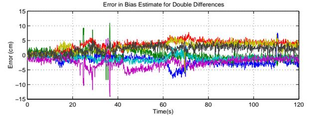
**Fig. 13:** Error in Bias Estimate for Double Difference Measurements, Frequent Re-Initialization with Null Space Algorithm, Data 2
