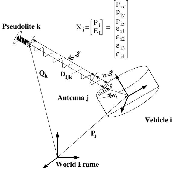
**Fig. 2:** Definition of the vehicle state and GPS measurements for the indoor formation flying testbeds.
