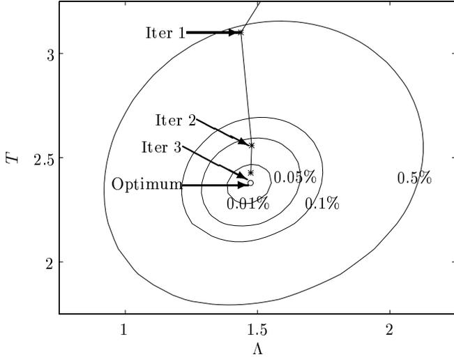
**Figure 3:** Contour plots of the  $\mathcal{H}_2$  cost overbounds as a function of the multiplier parameters over a refined region.
