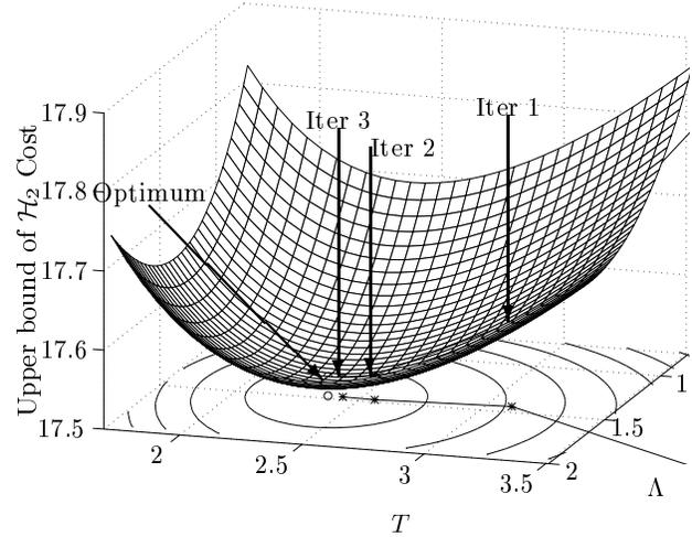
**Figure 4:** Mesh plots of the  $\mathcal{H}_2$  cost overbounds as a function of the multiplier parameters over a refined region.
