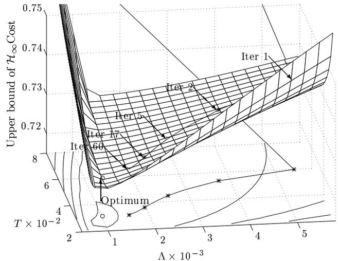
**Fig. 2:** Mesh plot of the  $\mathcal{H}_\infty$  cost overbounds as a function of the multiplier parameters ( $\Lambda$  and  $T$ ).
