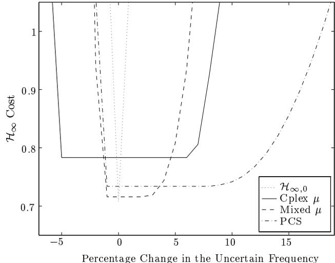
**Fig. 1:** Robust performance comparison for the complex  $\mu$ , mixed  $\mu$ , and Popov  $\mathcal{H}_\infty$  controller synthesis with  $\pm 1\%$  guaranteed stability bounds.
