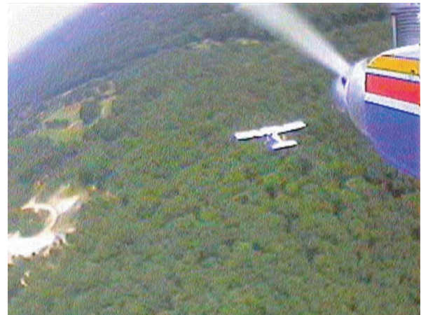
Figure 12. Aerial photo from the onboard camera during the autonomous rendezvous of two aircraft using timing control.
