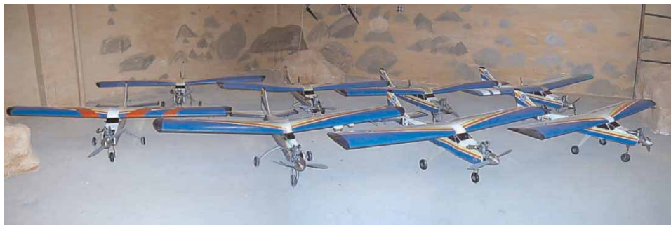
Figure 5. Fleet of eight identical Trainer 60 aircraft used in the multi-UAV testbed at MIT.
