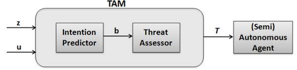
Fig. 1. High-level architecture of the TAM. The inputs of the TAM are the measurement history  $z$  of the  $\mathcal{OV}_s$  and the candidate control sequence  $u$  generated by the  $\mathcal{HV}$  planner. The IP computes the intention vector  $b$  for each  $\mathcal{OV}$ , used by the TA to identify the threat level  $\mathcal{T}$ .
