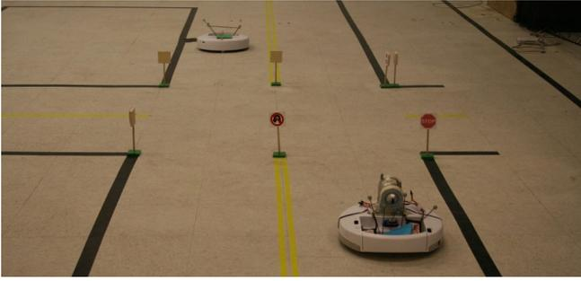
Fig. 2. The road network used for experiments. In this image, both a human-driven vehicle (front-right) and autonomous vehicle (back-left) are approaching a four-way, stop-sign intersection.
