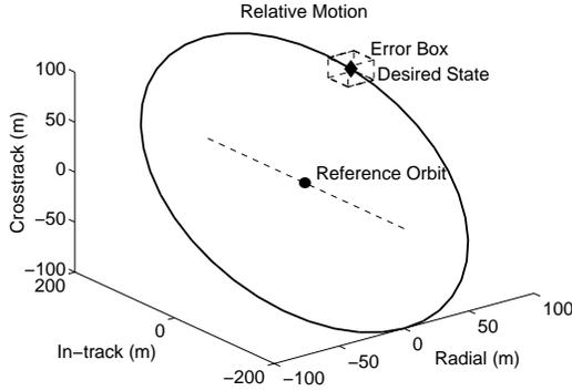
**Fig. 1:** Satellite motion relative to a reference orbit. Current position of the reference orbit is denoted with a circle, and the current desired relative position is with a diamond. An error box is centered on the diamond.
