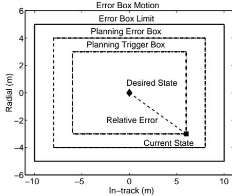
**Fig. 2:** In-plane view of error box. Three limits: plan trigger limit, planning error box constraint limit, hard performance (error box limit) constraint. The desired state is represented by the diamond while the current state is the square.
