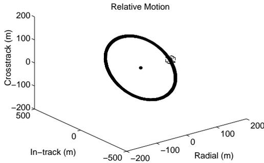
**Fig. 3:** Relative motion of satellite during the two week simulation. The circle represents the reference orbit and the diamond enclosed the box represents an example of the desired state and error box.
